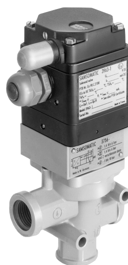
Bild 2: 3/2-way solenoid valve · Actuated on one side · With spring return mechanism · K_{VS} 4.3 · G 1/2 connection
