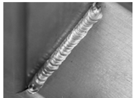
■ Fillet weld Function: HYPER.PULS with filler material
