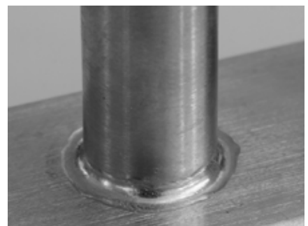
■ Circumferential weld Function: HYPER.PULS without filler material
