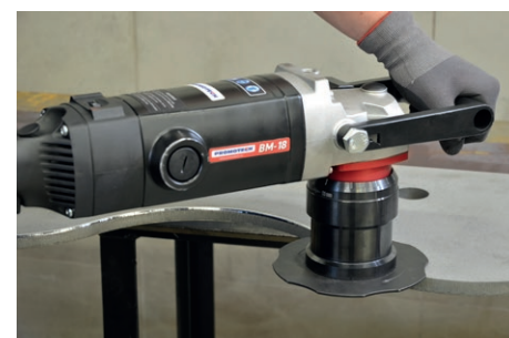
Rounding off curved edges
