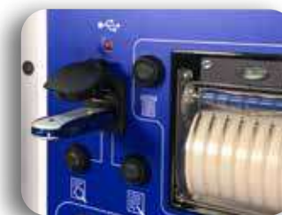
Multiple USB ports (4 in total) for backup, transfer and archiving of welding programmes and monitored data (USB stick supplied)
