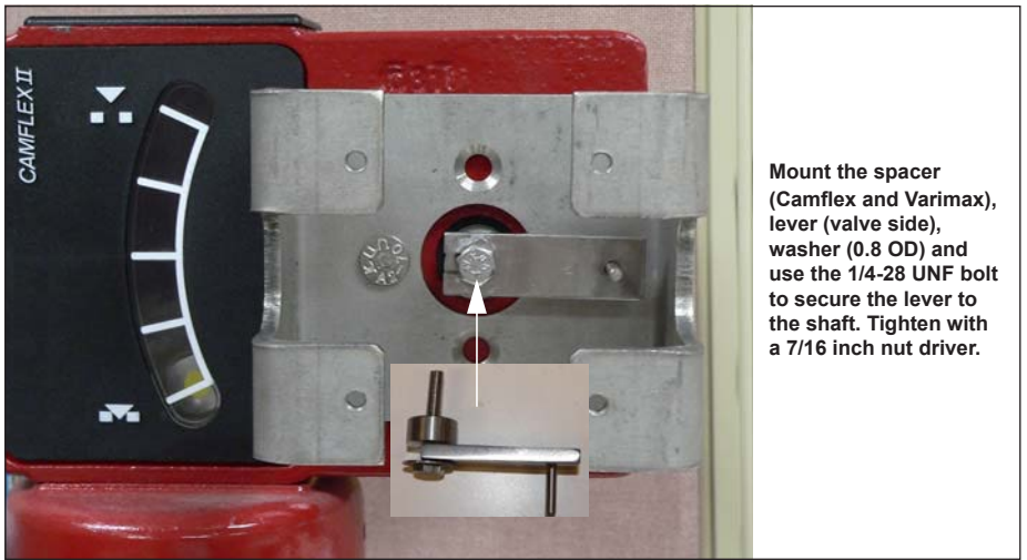
Figure 15 Attach Valve Side Lever to Valve
