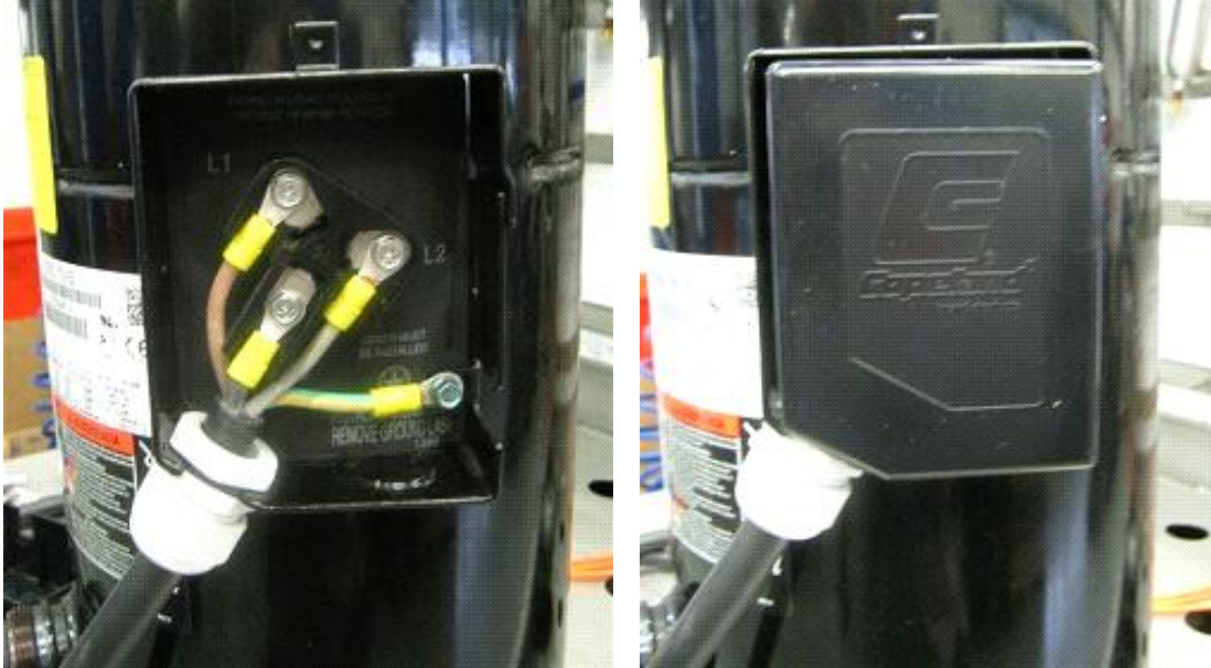
Figure 20: Electrical installation with cable glands, terminal box IP21
