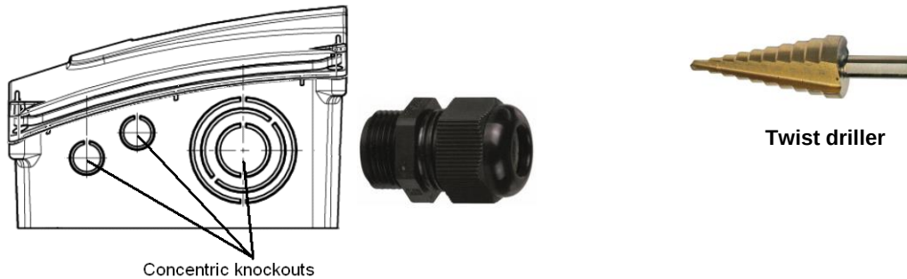
Figure 18: Knockouts on terminal box
