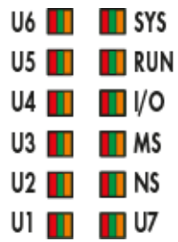
Figure 113: Indicating Elements for Fieldbus/System
