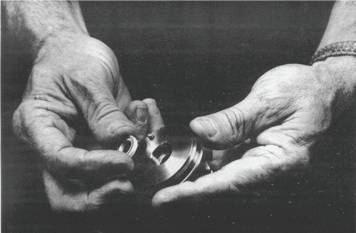
Figure 4-21 Installing Bal-Seal (20) in Piston Groove (18)
