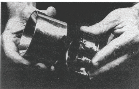
Figure 4-21 Installing Bal-Seal (20) in Piston Groove (18)
