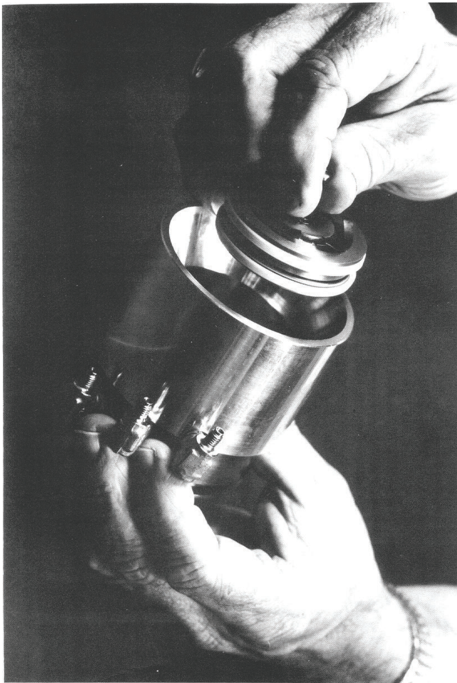
Figure 4-23 Inserting Piston Assembly (15 and 18) into Base (16)
