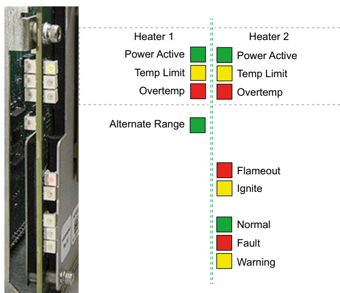
Figure 3-11 Base3DPM Status LEDs
