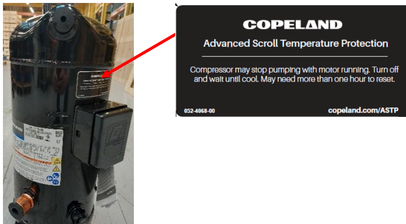
Figure 12: Scroll compressor with Advanced Scroll Temperature Protection (ASTP) sticker
