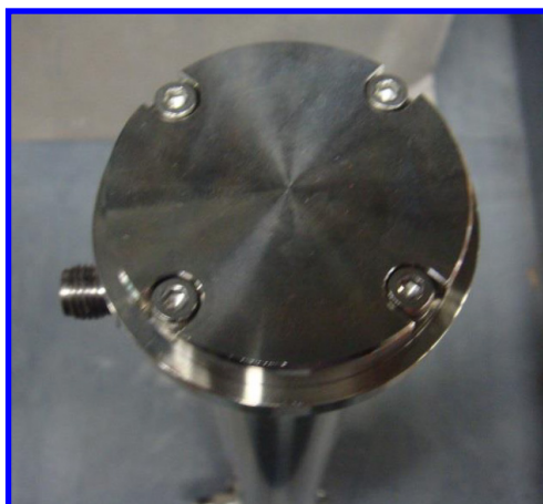
Bottom Cap – shown removed – with o-ring and Compression Spring.
