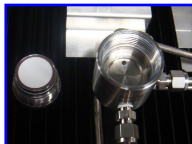
Filter cap—shown removed, at left—with o-ring and Membrane Filter installed in cap.
