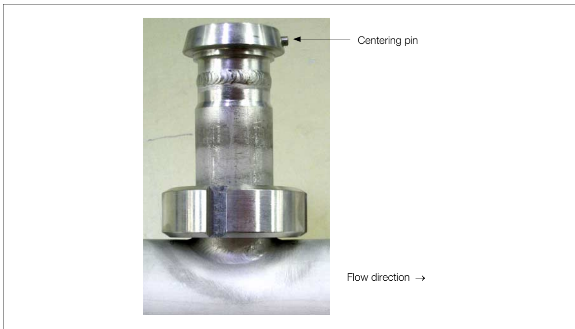
Bild 4-2 Weld-on adapter DIN11851 mounted to pipeline, centering pin right (outflow side)
